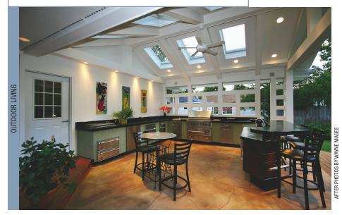
Custom concrete countertops feature internal steel reinforcement that increases their durability. Formed concrete backsplashes, also site-built, were designed to incorporate electrical outlets within their profile.
